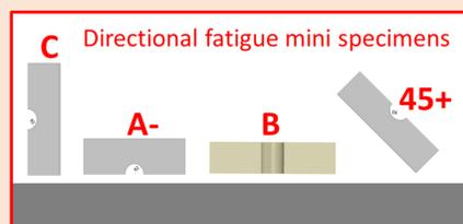
Miniaturized specimens divided into four different orientations produced to evaluate effect of build direction on fatigue performance of the material and to generate fatigue data useful for the part qualification phase.
