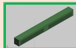
Process Calibration specimen for evaluation of inherent strains.
