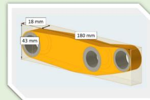
To perform optimization of the part, the geometry is divided in the "design space" where material is present but can be removed to achieve an optimal geometry, and the "non-design space", where material and geometry are fixed to guarantee necessary interfaces (bearing seats etc.), that define the boundary conditions
