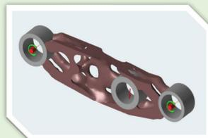
Topological optimization based on SIMP-algorithm (solid isotropic material with penalization) that attributes a varying density to each element. The optimization goal is defined in terms of minimization of the mass and global maximization of the stiffness. The solution respects imposed limits and is characterized by the best stiffness-to-weight ratio.
