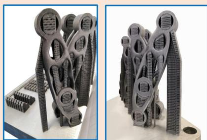
Optimized suspension arms printed according to two different orientations to investigate the differences introduced by dissimilar surface direction and supports position.
