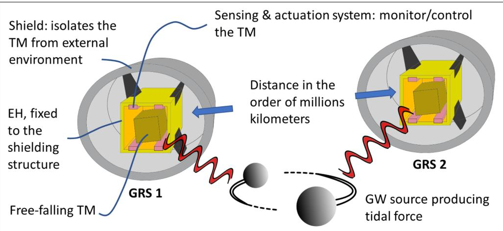
Concept of gravitational waves detection: measure the strain distance between a couple of free-falling TMs.
