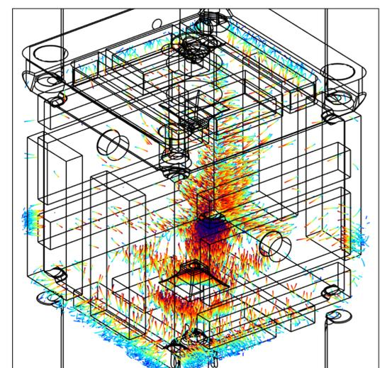
Screenshot of photoelectron trajectories inside the GRS. Light blue: slowest electrons; dark red: fastest electrons.
