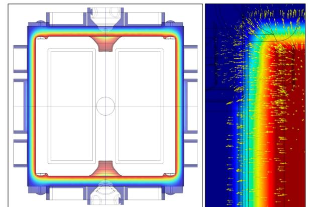
Left, electric potential inside the GRS. Right, detail near a TM vertex showing the electric field lines.
