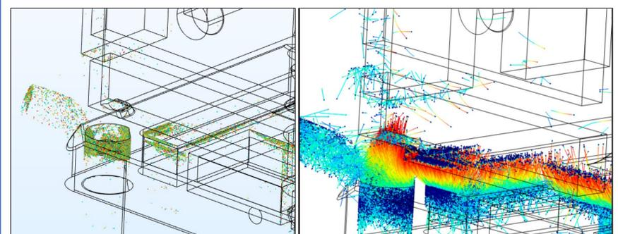
Largest part of the total photoelectrons is emitted from the numerous recesses (GAP) of the GRS. Left, emission points. Right, trajectories bent by the electric field.
