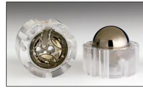
Gravity Probe – B uses spherical proof masses.
