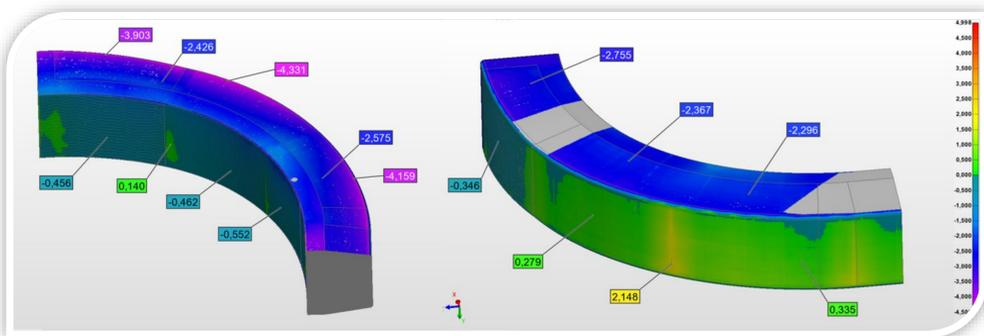
The initial deviations of the scan data from the nominal CAD show the optimization of the double pancakes stacking, (2.5-4 mm on top and bottom surfaces). The morphing and surfaces reconstruction respected the initial CAD topology, and adapted it onto the actual manufactured shape.
